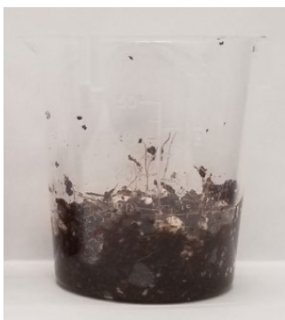
Test to determine EC of fresh media Slurry method 1:1 or 1:2
