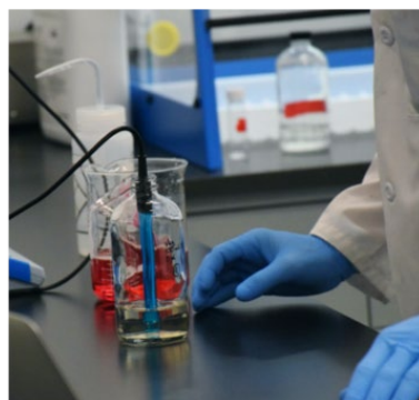
Test to determine EC of runoff Test EC of collected runoff after feeding
